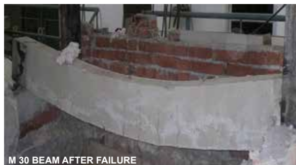
M 30 BEAM AFTER FAILURE
